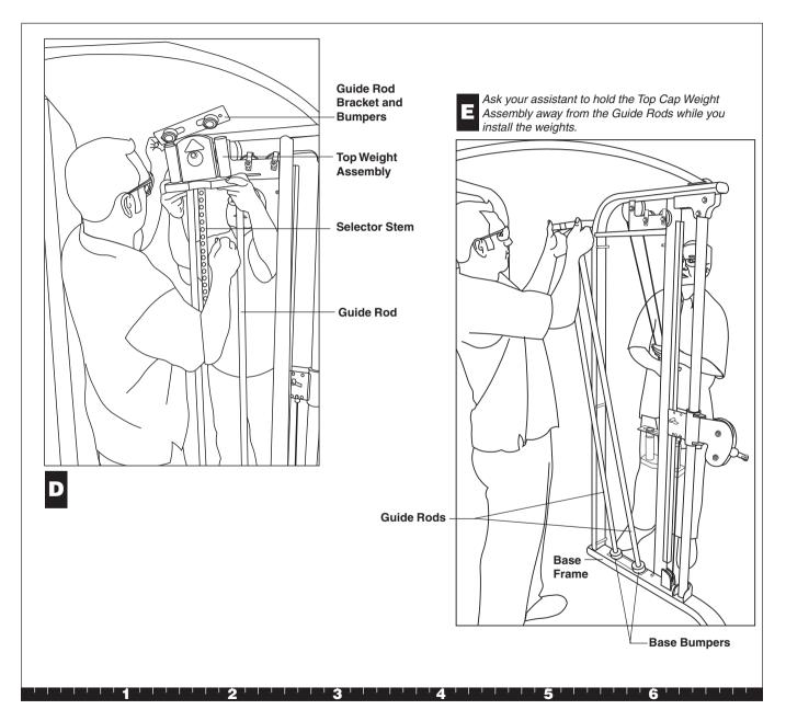
F. Hold the Guide Rods while your assistance replaces the Selector Stem and Top Weight Assembly.
